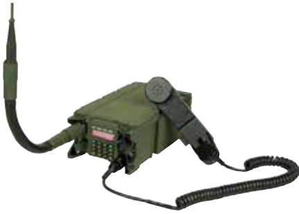
RT-1523 5 W manpack dismount configuration
