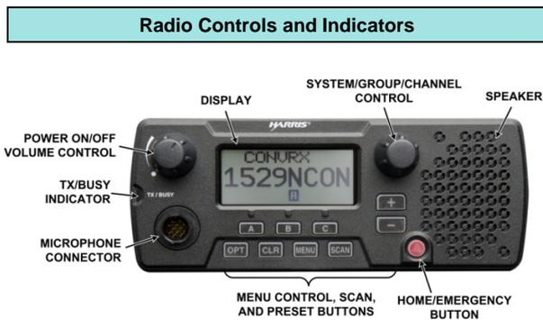
Figure 1: XG-25M Mobile Radio (Front View)
