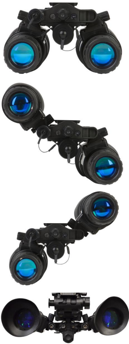
Figure 4. The images above show both the independent rotation and monocular standby state.
