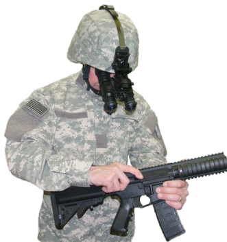
Figure 2. The F5032's close-focus capability of 25 cm (~9 inches) enhances the ability to read or repair weapons.
