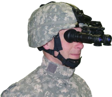
Figure 3. In addition to providing individual monocular functionality, the flip-out stow provides a significant improvement in stowed head-borne inertial loads and snag reduction.
